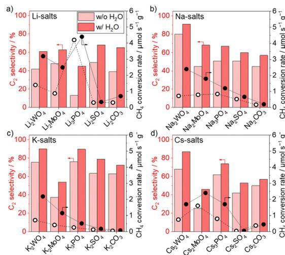
**Fig. 2** CH<sub>4</sub> conversion rate and C<sub>2</sub> selectivity of (a) Li-salt catalysts, (b) Na-salt catalysts, (c) K-salt catalysts, and (d) Cs-salt catalysts on SiO<sub>2</sub> for OCM at 850 °C with 10 kPa CH<sub>4</sub> and 1.7 kPa O<sub>2</sub> (balance Ar) using 0.2 g catalyst and 30–150 mL min<sup>-1</sup> flow extrapolated to 1% CH<sub>4</sub> conversion. Detailed results are listed in Table S2 (ESI<sup>†</sup>).
