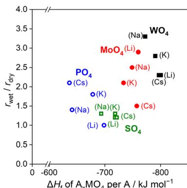
Fig. 3 Ratio of wet (1.7 kPa  $\text{H}_2\text{O}$  added) over dry (no additional  $\text{H}_2\text{O}$ )  $\text{CH}_4$  conversion rate as a function of formation enthalpy of the catalyst salt. Rates were determined at 1%  $\text{CH}_4$  conversion and 850 °C with 10 kPa  $\text{CH}_4$ , 1.7 kPa  $\text{O}_2$ , and balance Ar.
