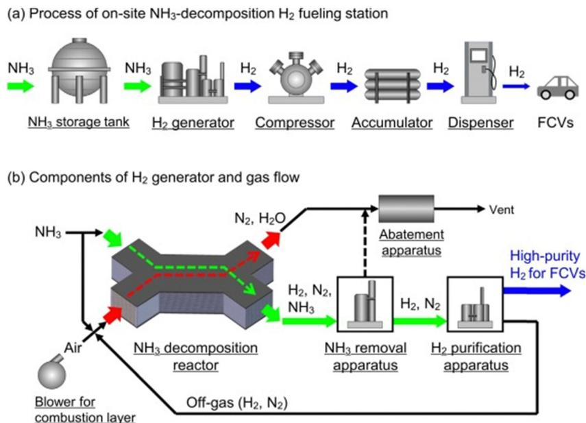
Fig. 1 Schemes of an on-site  $\text{NH}_3$ -decomposition  $\text{H}_2$  fuelling station (a) process of on-site  $\text{NH}_3$ -decomposition  $\text{H}_2$  fuelling station and (b) components of  $\text{H}_2$  generator and gas flow. (Reproduced from ref. 21. Copyright (2023), with permission from Elsevier).
