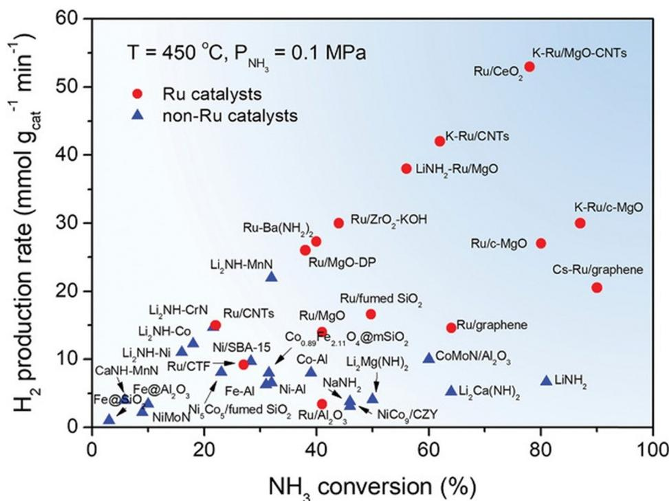
Fig. 4 Performance overview for NH<sub>3</sub> decomposition at 450–600 °C over various types of metal-supported catalysts. (Reproduced from ref. 50, with permission from John Wiley and Sons, copyright 2021). The aggregation states of metal presented in each catalyst are summarized in Table 1.
