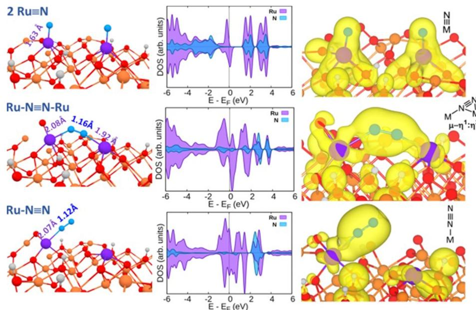
Fig. 14 Optimized structures, partial density of state and partial charge density of intermediate on Ru/MgO(111). (Reproduced from ref. 37. Copyright (2023), with permission from Nature).
