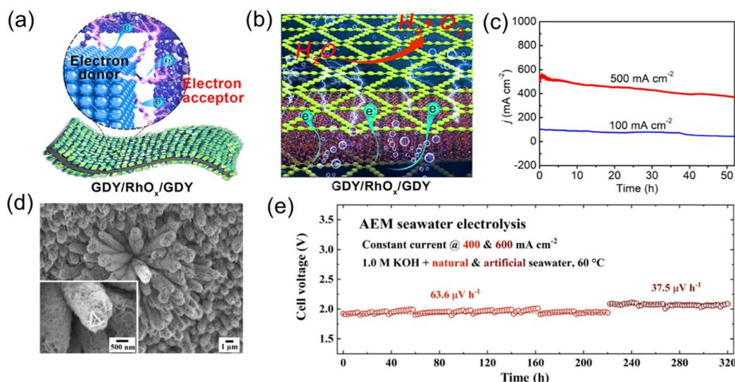
Fig. 4 (a) and (b) The efficient electron transfers from RhO<sub>x</sub> to GDY and the electron-rich GDY surface. (c) Chronoamperometry test of GDY/RhO<sub>x</sub>/GDY for overall seawater splitting at 500 and 100 mA cm<sup>-2</sup>.<sup>38</sup> Copyright © 2022 National Academy of Sciences. (d) FE-SEM of (Ni,Fe)O(OH)@NiCoS. (e) Cell voltage durability profiles at 400 and 600 mA cm<sup>-2</sup> feeding with alkaline seawater at 60 °C.<sup>39</sup> Copyright © 2023 Elsevier.
