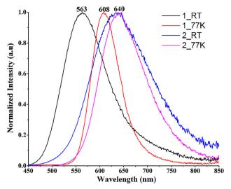
Fig. 5 Emission spectra in the solid state of  $\bf 1$  and  $\bf 2$  at 298 and 77 K (at  $\lambda_{\rm exc.}$  = 365 nm).
