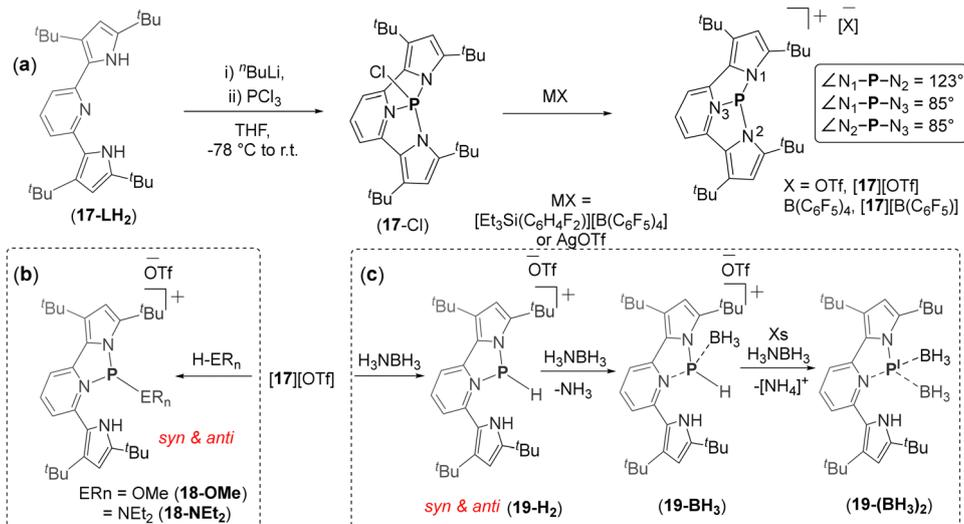
Fig. 9 (a) Synthetic scheme for the synthesis of  $[17][\text{OTf}]$  and  $[17][\text{B}(\text{C}_6\text{F}_5)_4]$ ; (b) activation of O–H, N–H bonds and (c)  $\text{H}_3\text{NBH}_3$  by  $[17][\text{OTf}]$ .
