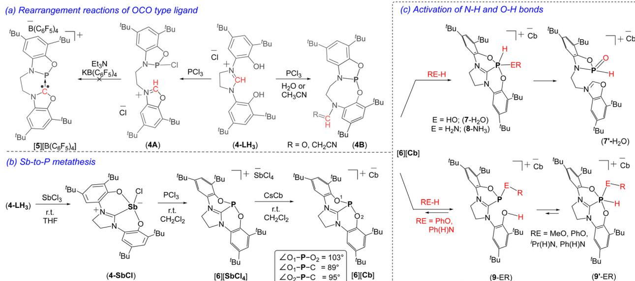
Fig. 5 Synthetic scheme showing: (a) phosphorus mediated rearrangement of an OCO type ligand; (b) Sb-to-P metathesis to prepare CSCP,  $[6][SbCl_4]$  and  $[6][Cb]$ ; (c) activation reactions of O-H and N-H bonds by  $[6][Cb]$ .
