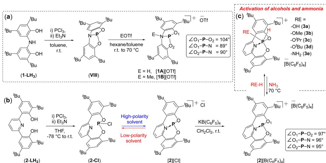
Fig. 4 Synthetic scheme for the synthesis of: (a) **[1A][OTf]** and **[1B][OTf]**; (b) **[2][B(C<sub>6</sub>F<sub>5</sub>)<sub>4</sub>]** and the activation of O–H and N–H bonds by **2**.
