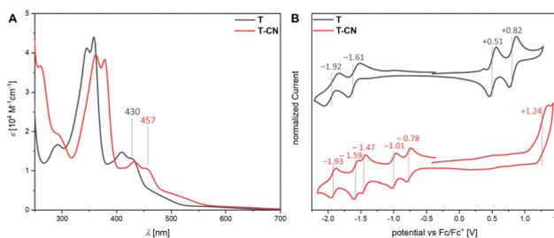
Fig. 3 (A) UV-Vis absorption spectra of **T** and **T-CN** ( $\text{CH}_2\text{Cl}_2$ ). (B) Cyclic voltammograms of **T** and **T-CN** ( $\text{CH}_2\text{Cl}_2$ ,  $n\text{Bu}_4\text{NPF}_6$  (0.1 M),  $c = 2$  mM,  $\nu = 149$   $\text{mV s}^{-1}$ ).
