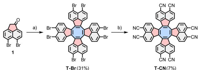
Scheme 1 Synthesis of octacyanated tridecacyclene **T-CN**. Reagents and conditions: (a)  $\text{TiCl}_4$ , *o*-DCB, 200 °C, 30 min; (b)  $[\text{Pd}_2(\text{dba})_3]$ , dppf,  $\text{CuCN}$ , 1,4-dioxane, 50 °C, 48 h. *o*-DCB = 1,2-dichlorobenzene, dba = dibenzylideneacetone, dppf = 1,1'-bis(diphenylphosphino)ferrocene.
