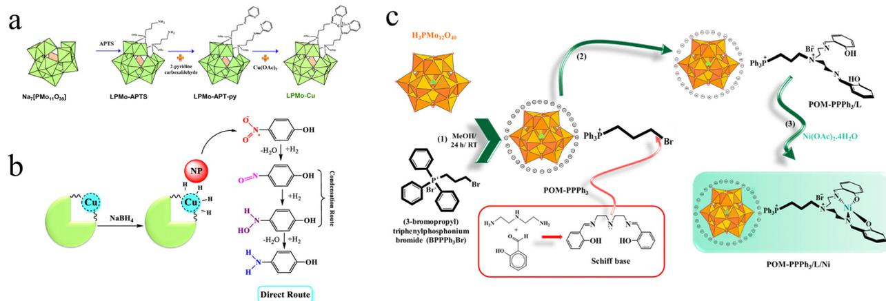
Fig. 8 (a) Schematic representation of the LPMo-Cu formation process and (b) proposed reaction path (direct path) for the reduction of the nitro group to the amino group. Adapted with permission.<sup>127</sup> Copyright 2023, American Chemical Society. (c) Proposed schematic of the route for the preparation of the POM-PPPh<sub>3</sub>/L/Ni nanocatalyst. Adapted with permission.<sup>48</sup> Copyright 2024, Royal Society of Chemistry.
