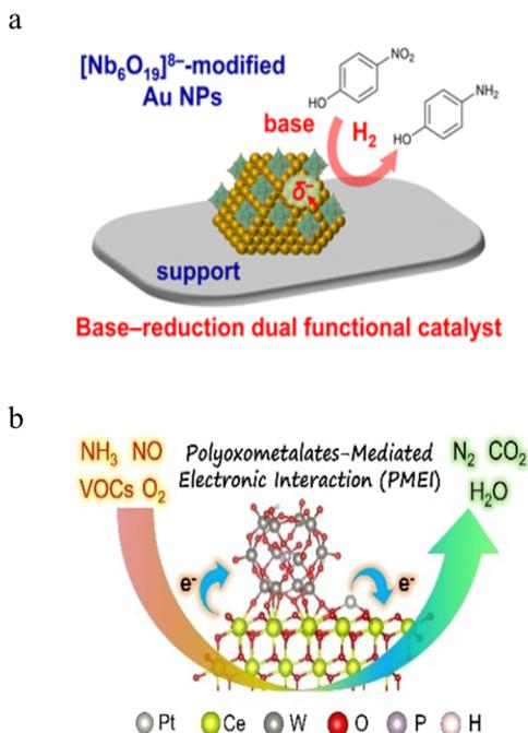
**Fig. 10** (a) Schematic diagram of the Nb<sub>6</sub>-Au/Al<sub>2</sub>O<sub>3</sub> catalyst for catalytic reduction of nitroaromatic hydrocarbons. Adapted with permission.<sup>134</sup> Copyright 2022, Royal Society of Chemistry. (b) Polyoxometalates-mediated electron interaction promotes the selective catalysis of Pt<sub>1</sub>/CeO<sub>2</sub> for nitric oxide. Adapted with permission.<sup>135</sup> Copyright 2024, Wiley-VHC.
