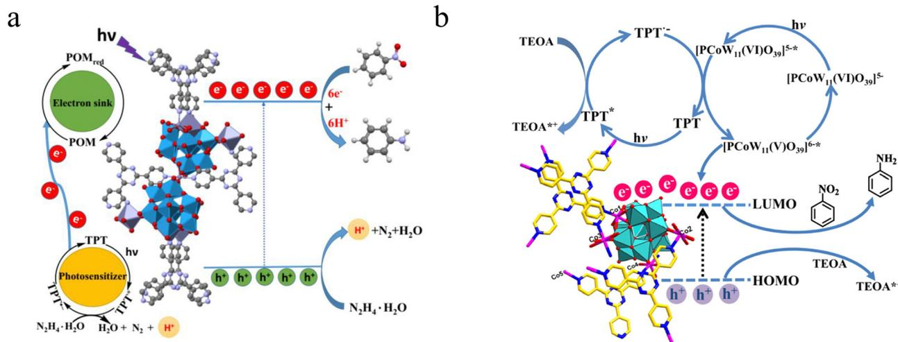
Fig. 12 (a) Photocatalytic diagram of the {CoW-TPT} for reduction of nitrobenzene. Adapted with permission.<sup>142</sup> Copyright 2022, American Chemical Society. (b) Photocatalytic diagram of the {ZnW-TPT} for reduction of nitroarenes. Adapted with permission.<sup>143</sup> Copyright 2022, American Chemical Society.
