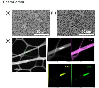
**Fig. 3** (a) SEM image of the EVOH/micro-NaCoHCF nanofibers. (b) SEM image of the EVOH/nano-NaCoHCF nanofibers. (c) EDX mapping of the EVOH/nano-NaCoHCF nanofibers.
