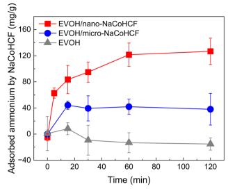
Fig. 4 Change of ammonium adsorption capacity of NaCoHCF in the EVOH/micro-NaCoHCF and EVOH/nano-NaCoHCF nanofibers (n = 3).
