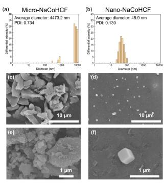
Fig. 2 (a) and (b) Intensity-weighted size distributions of the micro-NaCoHCF and nano-NaCoHCF particles measured by dynamic light scattering (DLS). The average diameters and polydispersion index (PDI) were calculated using the cumulant method. (c)-(f) SEM images of the synthesized NaCoHCF particles. (c) Micro-NaCoHCF with low magnification, (d) nano-NaCoHCF with low magnification, (e) micro-NaCoHCF with high magnification, and (f) nano-NaCoHCF with high magnification.
