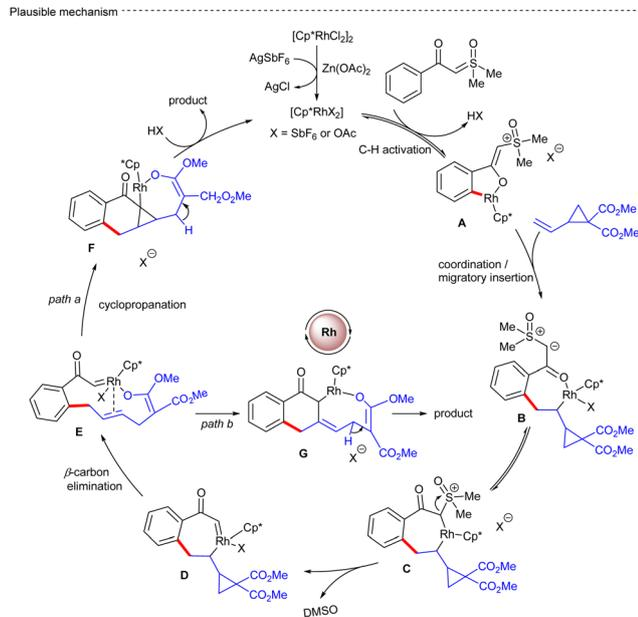
**Scheme 15** Rh-catalyzed sulfoxonium-ylide directed C-H/C-C functionalization with VCPs.
