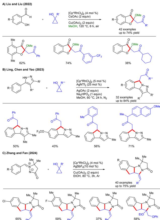
Scheme 28 Rh-catalyzed cascade annulation via C–H/C–C functionalization.
