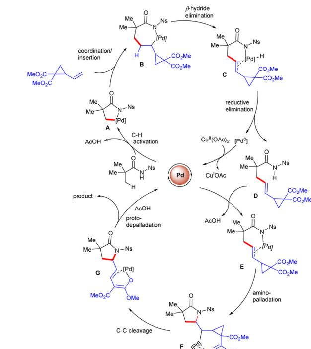
**Scheme 16** Pd-catalyzed sulfonamide directed C(sp<sup>3</sup>)-H/C-C functionalization with VCPs.
