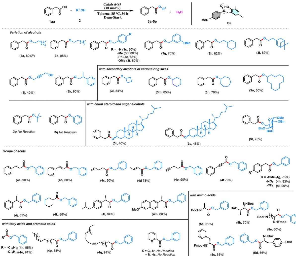
**Scheme 2** Substrate scope. Reaction conditions: **1aa** (1.0 equiv. 0.7 mmol), **2** (1.5 equiv. 1.09 mmol), catalyst **S5** (10 mol%) in toluene (2 ml) was refluxed in a Dean–Stark apparatus for 30 h. <sup>a</sup> Isolated yield.
