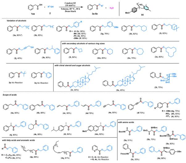
Scheme 2 Substrate scope. Reaction conditions: 1aa (1.0 equiv. 0.7 mmol), 2 (1.5 equiv. 1.09 mmol), catalyst \$5 (10 mol%) in toluene (2 ml) was refluxed in a Dean-Stark apparatus for 30 h. a Isolated vield.
