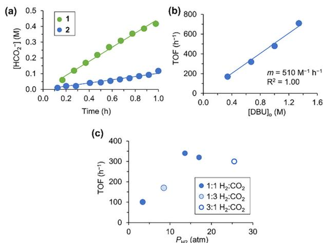
**Fig. 2** (a) Conversion of CO<sub>2</sub> to formate by **1** and **2**. Conditions: 0.5 mM/**2**, 600 mM DBU, 17 atm H<sub>2</sub>/17 atm CO<sub>2</sub> at 25 °C in CD<sub>3</sub>CN. (b) Plot of the DBU dependence on the TOF for **2** (17 atm H<sub>2</sub>/17 atm CO<sub>2</sub>, 25 °C). (c) Plot of the H<sub>2</sub> dependence on the TOF for **2** ([DBU]<sub>0</sub> = 0.61–0.67 M, 25 °C).
