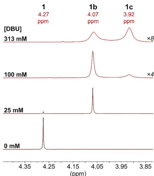
**Fig. 3** <sup>1</sup>H NMR spectrum (500 MHz, CD<sub>3</sub>CN, 25 °C) of the Cp resonance of **1** (25 mM) with varying [DBU]. Spectra with 100 and 313 mM DBU are magnified ×4 and ×8, respectively, due to significant broadening of the Cp signals.
