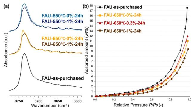
Fig. 1 Normalized FT-IR spectra (a) and water vapor adsorption isotherms (b) of as-purchased and representative treated FAU samples.
