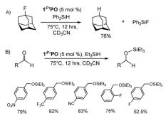
Catalytic applications of 1<sup>iPr</sup>PO: (A) hydrodefluorination of 1adamantyl fluoride and (B) hydrosilylation of electron-deficient aromatic aldehydes.
