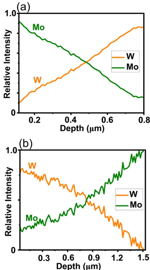
Fig. 3 Glow discharge optical emission spectroscopy (GDOES) plots revealing spatial changes in composition of Mo and W as a function of depth in deposited thin films. (a)  $\text{Mo}_x\text{W}_{1-x}\text{S}_2$  and (b)  $\text{W}_x\text{Mo}_{1-x}\text{S}_2$ .
