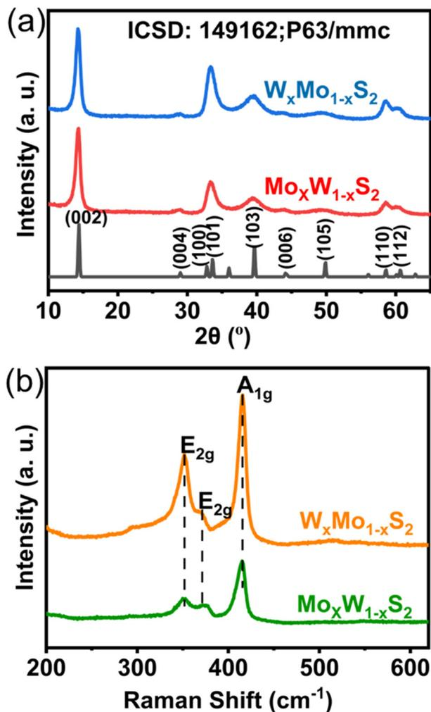
Fig. 1 (a) Grazing incidence powder X-ray diffraction (GI-XRD) patterns of  $\text{Mo}_x\text{W}_{1-x}\text{S}_2$  and  $\text{W}_x\text{Mo}_{1-x}\text{S}_2$  thin films compared to a standard 2H- $\text{MoS}_2$  powder pattern. (b) Raman Spectra of  $\text{Mo}_x\text{W}_{1-x}\text{S}_2$  and  $\text{W}_x\text{Mo}_{1-x}\text{S}_2$  thin films.
