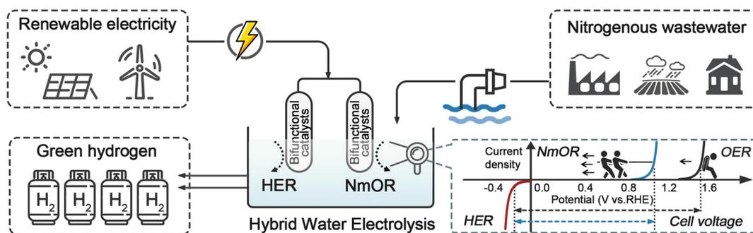
Fig. 1 Schematic of H<sub>2</sub> generation from renewable energy-powered HWE systems in nitrogenous wastewater.
