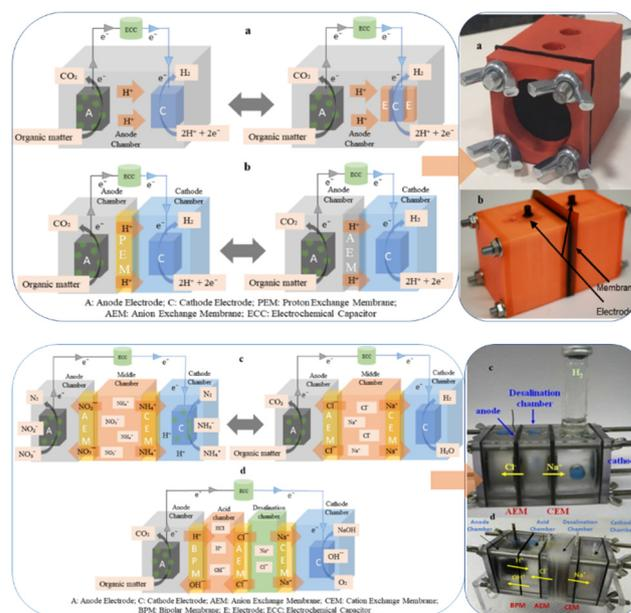
Fig. 2 A schematic and real images of MEC system forms categorized by application and compartment (a) SC-MEC and SC-MEC with sandwich C-electrode<sup>8</sup> (b) DC-MEC with PEM and DC-MEC with AEM<sup>8,45</sup> (c) three-chamber MEC<sup>46</sup> and (d) four chambers MEC.<sup>47,48</sup>
