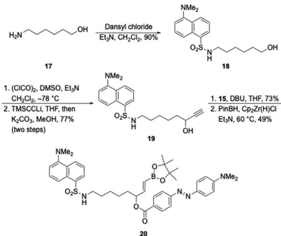
Scheme 4 Synthesis of an allylic-substituted latent fluorophore.
