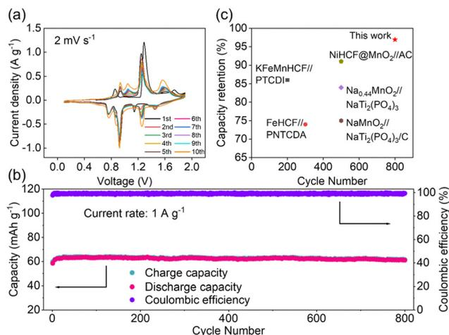
Fig. 6 Electrochemical performance of the Cu-HCF//P420 full cell. (a) Initial ten CV curves at  $2 \text{ mV s}^{-1}$ . (b) Cycling performance of the full cell at  $1 \text{ A g}^{-1}$ . (c) Capacity retention comparison graph.
