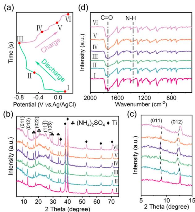
Fig. 5 (a) GCD curves of the P420 anode. Six SOC points were chosen. Point I: open-circuit potential state ( $\sim 0.14 \text{ V}$ ), point II: discharge to  $-0.5 \text{ V}$ , point III: discharge to  $-0.8 \text{ V}$ , point IV: charge to  $-0.3 \text{ V}$ , point V: charge to  $0 \text{ V}$ , and point VI: charge to  $0.2 \text{ V}$ . (b) XRD patterns under different SOC points. (c) Evolution of the (011) and (012) peaks. (d) FT-IR spectra showing C=O and N-H bands.
