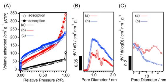
Fig. 2 (A)  $\text{N}_2$  adsorption–desorption isotherms of (a) Al-D4R-TEA, (b) Al-D4R-Py, and (c) Al-D4R-Pip. (B) and (C) Pore size distributions of (a) Al-D4R-Py and (b) Al-D4R-Pip (B: SF method, C: BJH method).
