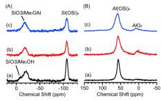
Fig. 1 (A)  $^{29}$ Si MAS NMR spectra and (B)  $^{27}$ Al MAS NMR spectra of (a) Al-D4R-TEA, (b) Al-D4R-Py, and (c) Al-D4R-Pip.
