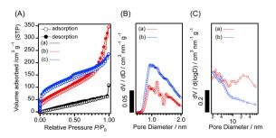
Fig. 2 (A) N<sub>2</sub> adsorption-desorption isotherms of (a) Al-D4R-TEA, (b) Al-D4R-Py, and (c) Al-D4R-Pip. (B) and (C) Pore size distributions of (a) Al-D4R-Py and (b) Al-D4R-Pip (B: SF method, C: BJH method).
