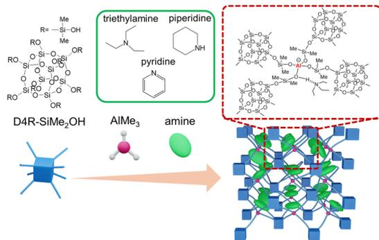
**Scheme 1** Synthesis of nanoporous aluminosilicates through a condensation reaction of dimethylsilanol-modified cage siloxane with  $\text{AlMe}_3$  in the presence of amines. In the dotted frame, triethylamine is shown as an example.
