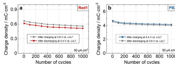
Fig. 4 Charge/discharge measurements over 1000 switching cycles for (a) **Red1** and (b) **PB2**, performed at 50  $\mu$ A cm<sup>-2</sup>.
