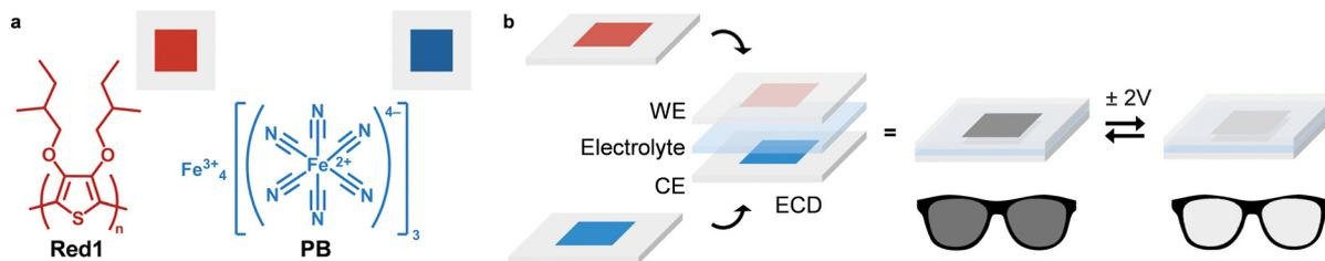
**Fig. 1** (a) Structures of **Red1** and **PB**; (b) schematic representation of the assembly of electrodes to provide a neutral-tint ECD and potential application in eyewear. WE = working electrode (**Red1**), CE = counter electrode (**PB**).
