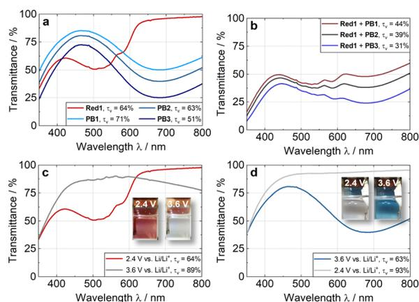
**Fig. 3** (a) UV-vis absorbance spectra of three different **PB** electrodes and (b) their combination with **Red1**; spectroelectrochemical characterization of the (c) **Red1** and (d) **PB2** electrodes with Li as CE/RE in 1 M LiTFSI/PC.
