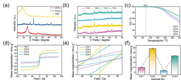
**Fig. 1** Characterization of the thin films. (a) Individual XRD patterns of each component in the TCF film; (b) XRD characterization of thin films TCF1-4; (c) thermogravimetric analysis of films TCF1-4 in air; (d) saturation magnetization of films TCF1-4; (e) coercivity and remanent magnetization of films TCF1-4; and (f) saturation magnetization of films TCF1-4.
