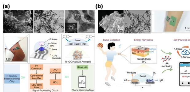
**Fig. 8** (a) Nonenzymatic sweat wearable UA sensor based on N-doped reduced graphene oxide/Au dual aerogels (copyright 2024, John Wiley and Sons).<sup>86</sup> (b) MA-based integrated wearable biofuel cell for self-powered epidermal sweat biomarker monitoring (copyright 2023, American Chemical Society).<sup>87</sup>
