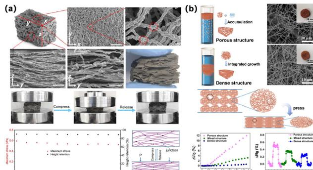
Fig. 3 (a) Morphology and mechanical properties of NNWAs (copyright 2022, John Wiley and Sons).<sup>51</sup> (b) Controlled fabrication of Cu NW aerogels with different structures and pressure-response for aerogels (copyright 2017, American Chemical Society).<sup>52</sup>
