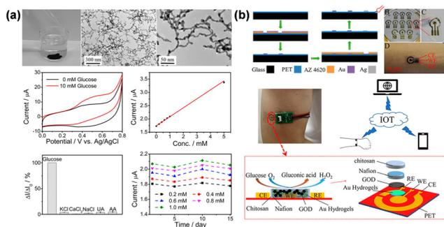
**Fig. 6** Integrating highly porous and flexible Au aerogels with soft-MEMS technologies for high-performance wearable biosensing.<sup>84</sup> (a) The optical image, micromorphology and electrochemical test results of Au aerogels. (b) Manufacturing processes of MEMS electrodes (copyright 2021, American Chemical Society).
