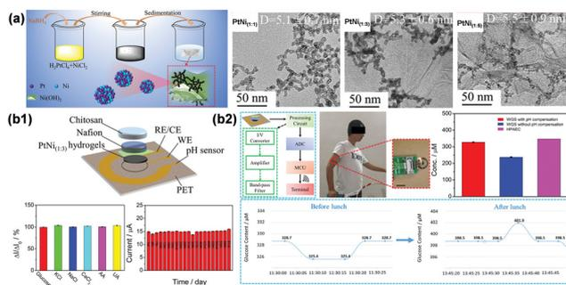
**Fig. 7** (a) Synthesis, morphology and structure of the PtNi<sub>(1:X)</sub> dual aerogels. (b1) Schematic illustration, the selectivity and the long-term stability of the PtNi<sub>(1:3)</sub> aerogel-based sensing chip. (b2) Wearable application of the PtNi<sub>(1:3)</sub> dual aerogel-based glucose sensor (copyright 2023, John Wiley and Sons).<sup>85</sup>
