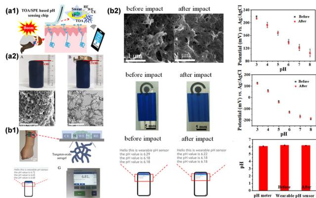
Fig. 9 Shock-resistant wearable pH sensor based on tungsten oxide aerogels (copyright 2024, Elsevier).<sup>89</sup>
