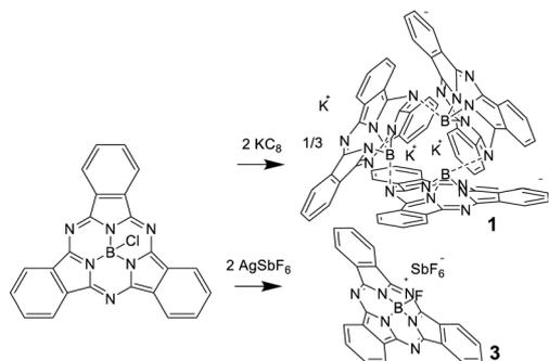
Scheme 1 Synthetic route to  $(\text{K}^+[\text{sub}^{\text{PcB}}])_3$  (**1**) and  $[\text{sub}^{\text{PcBF}}][\text{SbF}_6]$  (**3**).
