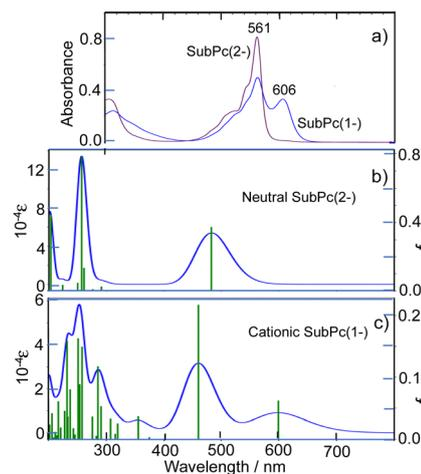
Fig. 4 (a) UV-visible absorption spectra of <sup>sub</sup>PcBF (**2**) (purple line) and [<sup>sub</sup>PcBF][SbF<sub>6</sub>] (**3**) (blue line) in THF. Calculated absorption spectra of (b) neutral and (c) mono-cationic <sup>sub</sup>PcB. Note scale difference of *f* and *ε* between (b) and (c). DFT and TDDFT calculations were carried out using the CAM-B3LYP functional with 6-31+G(d,p) basis sets.
