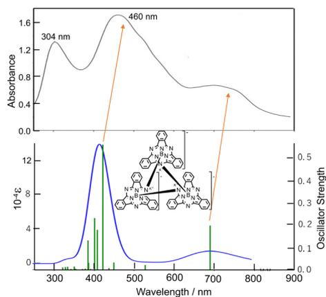
Fig. 3 (top) Absorption spectrum of **1** in THF, and (bottom) that of calculated spectrum. Due to the large molecular size, energies in the region above 310 nm were not calculated. DFT and TDDFT calculations were carried out using the CAM-B3LYP functional with 6-31+G(d,p) basis sets.
