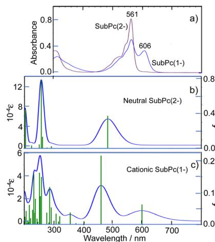
Fig. 4 (a) UV-visible absorption spectra of <sup>sub</sup>PcBF (**2**) (purple line) and [<sup>sub</sup>PcBF][SbF<sub>6</sub>] (**3**) (blue line) in THF. Calculated absorption spectra of (b) neutral and (c) mono-cationic <sup>sub</sup>PcB. Note scale difference of  $f$  and  $\epsilon$  between (b) and (c). DFT and TDDFT calculations were carried out using the CAM-B3LYP functional with 6-31+G(d,p) basis sets.
