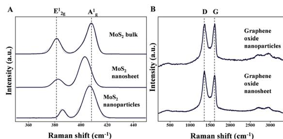
Fig. 3 Raman analysis of (A) MoS<sub>2</sub> bulk, nanosheets, and nanoparticles as well as (B) GO nanosheets and nanoparticles.
