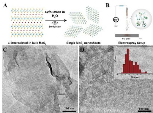
**Fig. 1** (A) A schematic of the preparation of MoS<sub>2</sub> nanosheets from bulk MoS<sub>2</sub> through wet chemical synthesis. (B) Schematic of the electro spray set-up. (C) Transmission electron microscopy (TEM) image showing the MoS<sub>2</sub> nanosheets synthesized by wet chemical synthesis. (D) Large area TEM image of MoS<sub>2</sub> nanoparticles formed by ambient electro spray. The inset shows the particle size distribution of electro sprayed MoS<sub>2</sub>.
