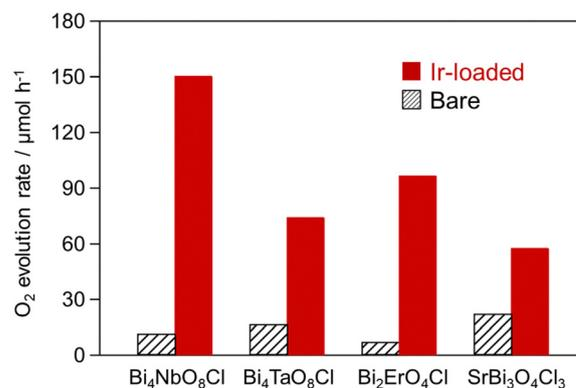
Fig. 5 Initial  $\text{O}_2$  evolution rate of oxyhalides loaded with or without Ir species *via* ADS method. These reactions were performed in aqueous  $\text{AgNO}_3$  solution (8 mM, 100 mL) containing the photocatalyst powder (0.1 g) under visible light irradiation ( $\lambda > 400$  nm) from a 300-W Xe-arc lamp.
