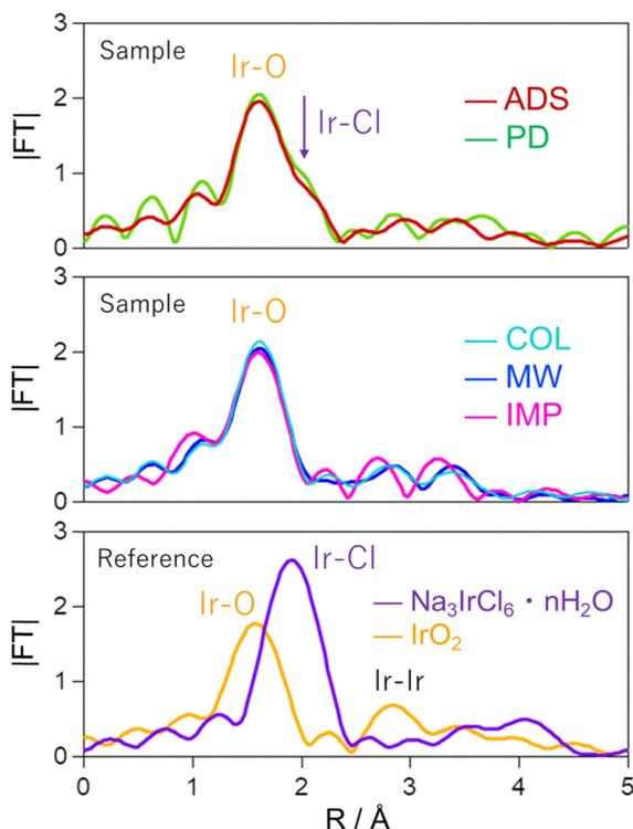
Fig. 4 Fourier-transformed Ir  $L_{3\text{-edge}}$  EXAFS spectra of  $\text{Bi}_4\text{NbO}_8\text{Cl}$  loaded with Ir species *via* various methods (COL, MW, IMP, PD, and ADS), along with those of reference samples.
