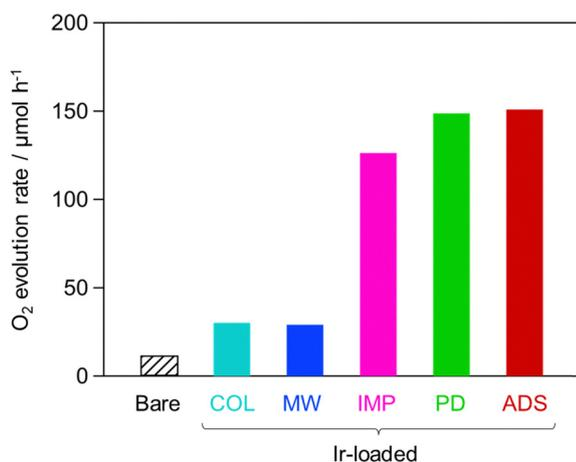
Fig. 2 Initial  $\text{O}_2$  evolution rate of  $\text{Bi}_4\text{NbO}_8\text{Cl}$  loaded with Ir species *via* various methods (COL, MW, IMP, PD, and ADS), along with that of bare  $\text{Bi}_4\text{NbO}_8\text{Cl}$ . These reactions were performed in aqueous  $\text{AgNO}_3$  solution (8 mM, 100 mL) containing the photocatalyst powder (0.1 g) under visible light irradiation ( $\lambda > 400$  nm) from a 300-W Xe-arc lamp.
