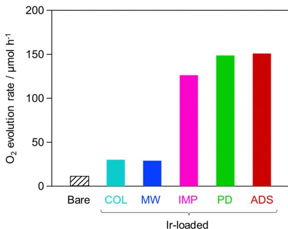
Fig. 2 Initial  $\text{O}_2$  evolution rate of  $\text{Bi}_4\text{NbO}_8\text{Cl}$  loaded with Ir species *via* various methods (COL, MW, IMP, PD, and ADS), along with that of bare  $\text{Bi}_4\text{NbO}_8\text{Cl}$ . These reactions were performed in aqueous  $\text{AgNO}_3$  solution (8 mM, 100 mL) containing the photocatalyst powder (0.1 g) under visible light irradiation ( $\lambda > 400$  nm) from a 300-W Xe-arc lamp.
