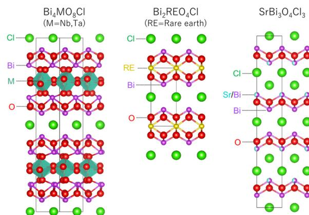
Fig. 1 Crystal structures of Sillén(-Aurivillius)-type layered oxyhalide photocatalysts: Bi<sub>4</sub>MO<sub>8</sub>Cl (M = Nb, Ta), Bi<sub>2</sub>REO<sub>4</sub>Cl (RE = rare earth), and SrBi<sub>3</sub>O<sub>4</sub>Cl<sub>3</sub>.
