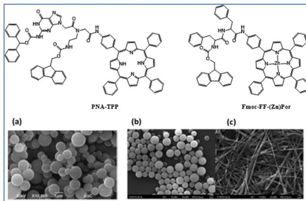
Fig. 2 Chemical nanostructures of self-assembled porphyrins and SEM images of (a) **PNA-TPP** CH<sub>2</sub>Cl<sub>2</sub>–EtOH, 2 : 8 (7 mM), (b) **Fmoc-FF-(Zn)Por** THF/MeOH, 2 : 8 (1 mM), and (c) **Fmoc-FF-(Zn)Por** CH<sub>2</sub>Cl<sub>2</sub>/Hept, 1 : 1 (1 mM). Reproduced from ref. 63 with permission from Royal Society of Chemistry, copyright 2019.
