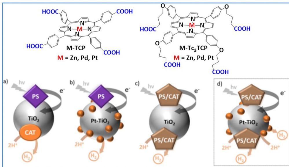
Fig. 5 Chemical structures of porphyrin molecules **M-TCP**, **M-Tc<sub>3</sub>TCP** adsorbed onto TiO<sub>2</sub> nanoparticles, (a) **PS** and **CAT** on TiO<sub>2</sub> nanoparticles, (b) **PS** onto Pt-TiO<sub>2</sub> nanoparticles, (c) **PS-CAT** onto TiO<sub>2</sub> nanoparticles, and (d) **PS-CAT** onto Pt-TiO<sub>2</sub> nanoparticles. Reproduced from ref. 72 with permission from Royal Society of Chemistry, copyright 2023.
