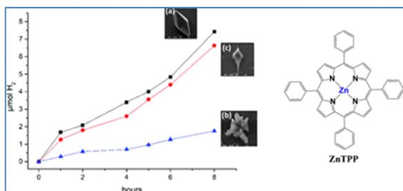
Fig. 4 Photocatalytic hydrogen production of ZnTPP with (a) octahedral (THF/MeOH 1:4), (b) “flower” (CHCl<sub>3</sub>/MeOH 1:4), and (c) “manta-ray” (Tol/MeOH 1:4) structures, in the presence of Pt nanoparticles. Reproduced from ref. 66 with permission from Royal Society of Chemistry, copyright 2022.
