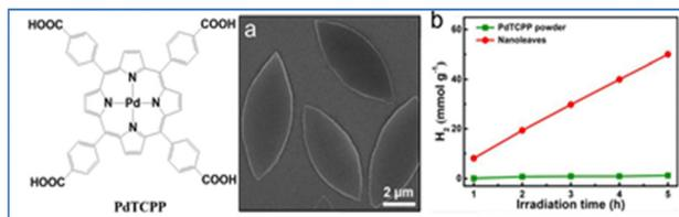
Fig. 3 Chemical structure of PdTCPP, (a) SEM image of nanoleaves, and (b) photocatalytic H<sub>2</sub> production of the commercial PdTCPP powder and nanoleaves without cocatalysts. Reproduced from ref. 65 with permission from American Chemical Society, copyright 2022.
