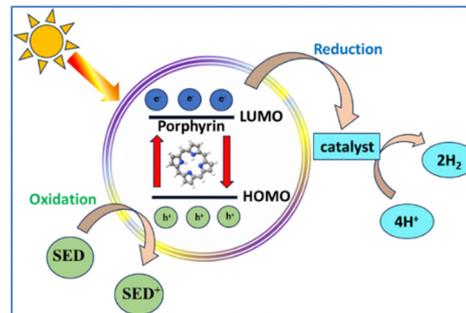
Scheme 2 Simplified scheme of half-cycle photochemical  $H_2$  evolution.
