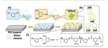
Fig. 6 (a) Schematic representation of preparation of membranes. (b) Schematic representation of the cages and openings of MIL-101(Cr). (c) IP process.<sup>59</sup>
