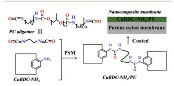
Fig. 11 A schematic illustration of preparing a CuBDC-NH2/PU nanocomposite membrane with an isocyanate-terminated PU oligomer. Adapted from ref. 25 with permission from the Elsevier.
