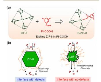
Fig. 18 Schematic illustration of (a) chemical reaction between ZIF-8 and PI-COOH to give rise to the etching of ZIF-8 nanoparticles in the PI-COOH matrix and (b) interface structure and gas transportation in ZIF-8 and E-ZIF-8 based hybrid membranes. Adapted from ref. 78 with permission from the Elsevier.
