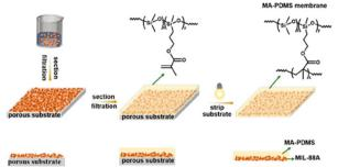
Fig. 10 Schematic drawing of the fabrication of the asymmetrical MIL-88A/MA-PDMS MMM. Reprinted adapted with permission from ref. 27. Copyright 2023 American Chemical Society
