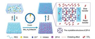
Fig. 13 Schematic illustration of the ZIF/PEO membrane preparation. Adapted from ref. 70 with permission from the John Wiley and Sons.
