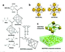
Fig. 7 (a) The synthetic route and structures of UiO-66-NH2, UiO-66-MA and MOF/PEO MMM. (b) Simulated crystal structures of UiO-66-NH2 and UiO-66-MA. (c) 3D structural illustration of the MOF/PEO MMM membrane (octahedrons represent UiO-66-MA particles; cylindrical wires represent PEO molecular chains).<sup>61</sup>
