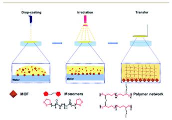
Fig. 9 Illustration of the preparation of oriented MOF polymer films.<sup>26</sup>
