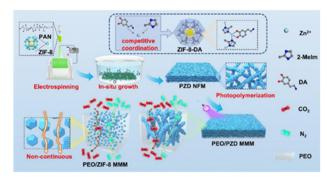
Fig. 14 Schematic diagram of the preparation and separation mechanism of PEO/PZD MMM. Adapted from ref. 74 with permission from the Elsevier.
