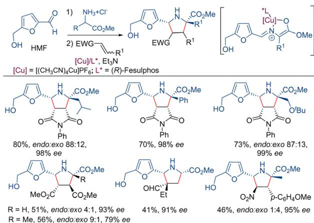
**Scheme 25** Cycloaddition between HMF derived-iminoesters and activated olefins.
