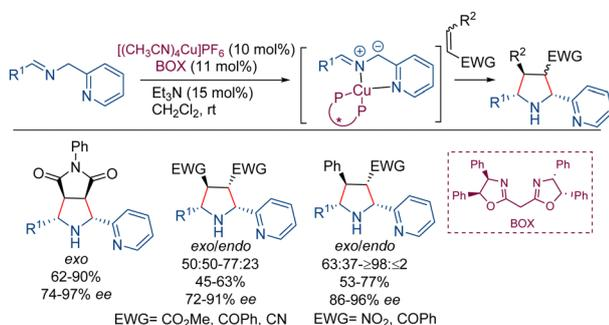
**Scheme 13** Intermolecular (3+2) cycloaddition between *N*-(2-pyridylmethyl)imines and different dipolarophiles.
