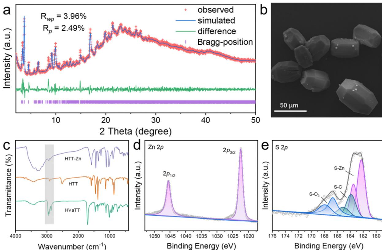
Fig. 2 (a) Rietveld refinement of the experimental PXRD pattern of **HTT-Zn** ( $R_{wp} = 3.96\%$ ;  $R_p = 2.49\%$ ). (b) SEM images of **HTT-Zn**. (c) FT-IR spectra of HVaTT, HTT and **HTT-Zn**. High-resolution XPS spectra of (d) Zn 2p, and (e) S 2p of **HTT-Zn**.
