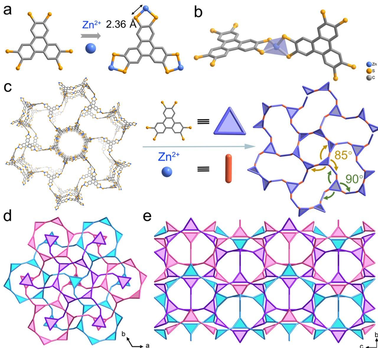
**Fig. 1** (a) Self-assembly of HTT<sup>6-</sup> and Zn(II) ions; (b) coordination environment of the Zn(II) centre; (c) 3D framework and topological network of **HTT-Zn**; representation of the 3-fold interpenetration network of **HTT-Zn** along the (d)  $c$ -axis and (e)  $a$ -axis directions.
