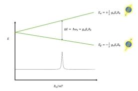
Fig. 5 Magnetic field dependence of the energy of the two spin states  $m_{\rm s}=+1/2~(\alpha~{\rm state})$  and  $m_{\rm s}=-1/2~(\beta~{\rm state})$  of the unpaired electron (Zeeman effect). The resonance phenomenon originates from the absorption of microwave energy that matches the energy difference  $\Delta E$  between the two  $m_{\rm e}$  states.
