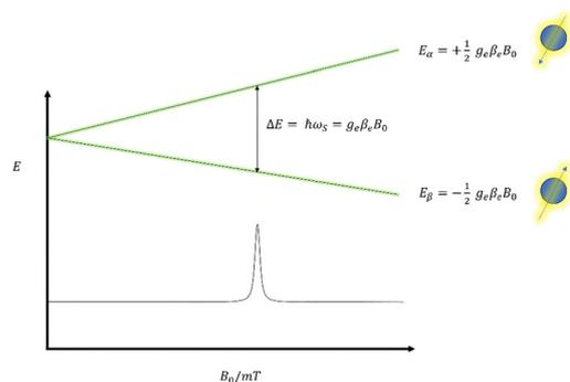
Fig. 5 Magnetic field dependence of the energy of the two spin states  $m_s = +1/2$  ( $\alpha$  state) and  $m_s = -1/2$  ( $\beta$  state) of the unpaired electron (Zeeman effect). The resonance phenomenon originates from the absorption of microwave energy that matches the energy difference  $\Delta E$  between the two  $m_s$  states.
