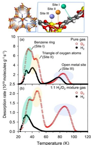
Fig. 3 (Top) Structural representation of the imidazole-based MOF-74 altogether with its theoretical adsorptive sites and (down) the thermal desorption spectra for pure gas and 1 : 1 H<sub>2</sub>/D<sub>2</sub> mixture gas at an exposure temperature of 25 K. Adapted with permission from ref. 43 Copyright 2017 American Chemical Society.
