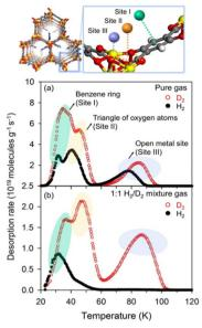
Fig. 3 (Top) Structural representation of the imidazole-based MOF-74 altogether with its theoretical adsorptive sites and (down) the thermal desorption spectra for pure gas and 1:1 H<sub>2</sub>/D<sub>2</sub> mixture gas at an exposure temperature of 25 K. Adapted with permission from ref. 43 Copyright 2017 American Chemical Society.
