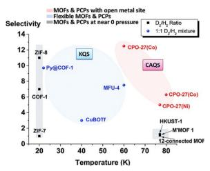
Fig. 1 Selectivity of hydrogen isotope adsorption (D2 over H2) for several porous frameworks as a function of working temperature. Reproduced from ref. 10 with permission from Wiley-VCH.
