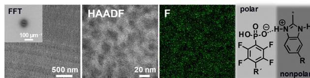
Fig. 2 Nanostructure analysis of PWN40-S blend membrane cross-section stained with Ba<sup>2+</sup>. HAADF-STEM images and diffractogram for nanostructure size determination with corresponding fluorine EDX spectrum and simplified chemical structure with crosslinking and assignment of polar and nonpolar segments.
