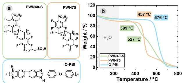
Fig. 1 (a) Chemical structures of PWN40-S, PWN75 and OPBI. (b) Thermogravimetric analysis of the pristine polymers with the assigned onset decomposition temperatures (heating rate: 10 K min<sup>-1</sup>, carrier gas: synthetic air).
