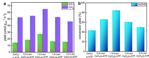
Fig. 4 Photocatalytic properties of various photocatalysts: (a) production yield of CO and CH<sub>4</sub>, and (b) conversion yield of ArCHO.
