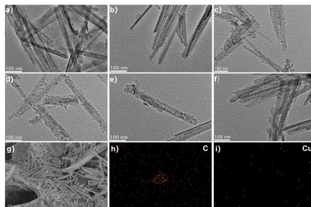
Fig. 2 TEM images of (a) ATP, (b) p-ATP, (c) CeO<sub>2</sub>/p-ATP, (d) 0.5-Lacc/CeO<sub>2</sub>/p-ATP, (e) 1.0-Lacc/CeO<sub>2</sub>/p-ATP and (f) 2.0-Lacc/CeO<sub>2</sub>/p-ATP. (g) SEM image, (h) and (i) EDX elemental mapping of 1.0-Lacc/CeO<sub>2</sub>/p-ATP.
