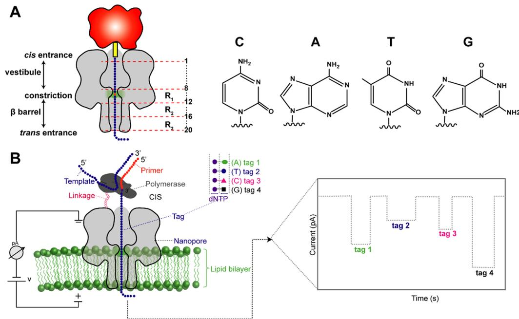
Fig. 8 Nanopore-based DNA sequencing. (A) The structure of  $\alpha$ -HL nanopores. R1, R2 and R3 represent the three base-recognition sites within the  $\beta$ -barrel domain. (B) The principle of nanopore-based single-molecule DNA sequencing using nucleotides with different polymer tags.
