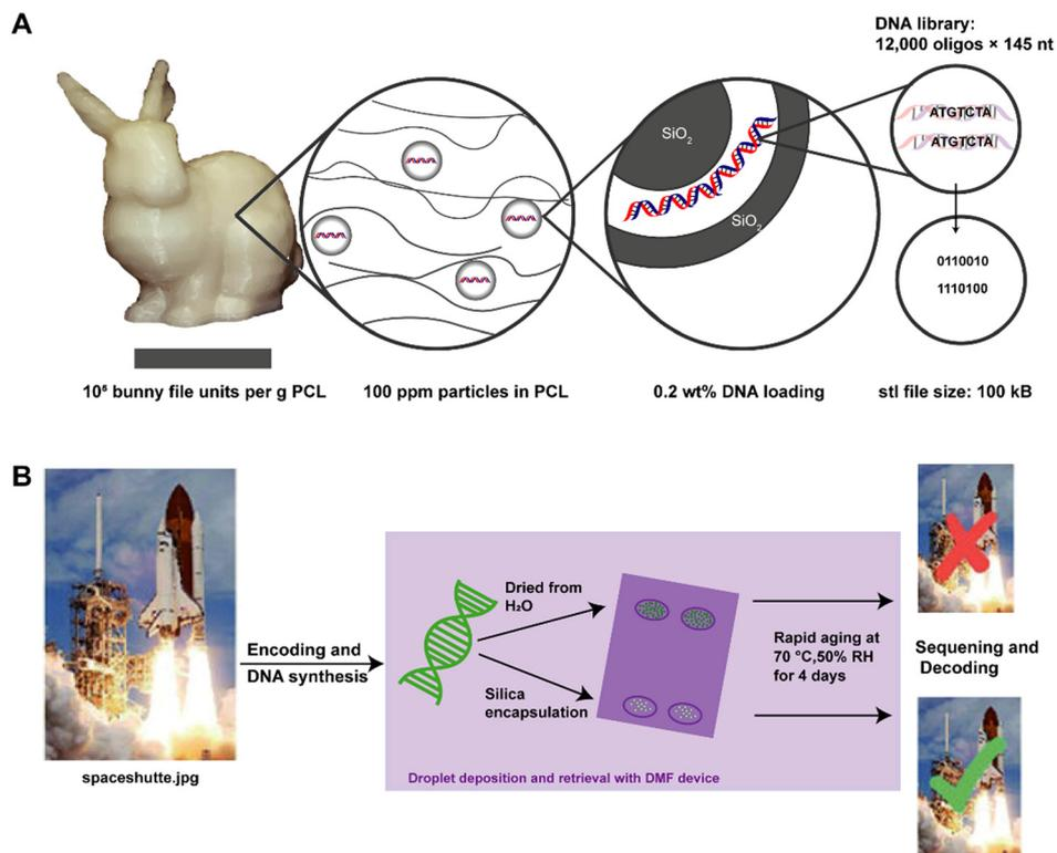
**Fig. 5** Strategies of *in vitro* long-term DNA data storage. (A) Schematic architecture of the 3D-printed Stanford Bunny, which contained the encapsulated DNA library. Reproduced from ref. 81 with permission from Springer Nature, copyright 2020. (B) Overview of digital microfluidics (DMF)-compatible silica nanoparticles encapsulating the DNA library for DNA data storage. Reproduced from ref. 82 with permission from Wiley, copyright 2022.
