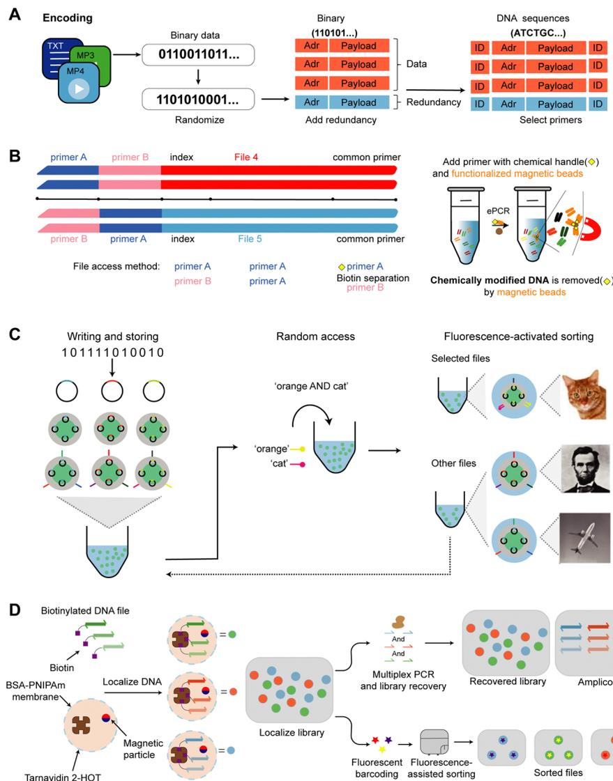
**Fig. 7** Random access in DNA data storage. (A) Design a primer library for PCR-based random access. (B) Using nested, hierarchical primer for addresses. (C) Silica capsules with dye-labelled orthogonal barcodes used to select the specific data by fluorescence-activated sorting. Reproduced from ref. 95 with permission from Springer Nature, copyright 2021. (D) Thermo-responsive proteinosomes using fluorescence-assisted sorting for repeated access in DNA data storage.
