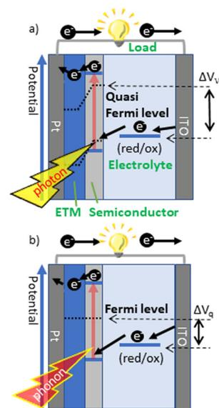
Fig. 5 Schematic image of the output potential by (a) photoexcitation and (b) thermal excitation. ETM: electron transport material<sup>43</sup> (Copyright © 2020 The Chemical Society of Japan).
