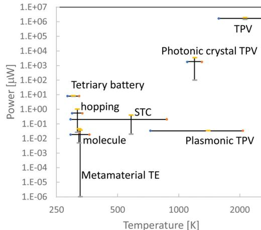
Fig. 1 The power generation temperature and maximum output power of thermal energy conversion technology at isothermal temperature. TPV: thermophotovoltaic energy conversion. STC: semiconductor-sensitized thermal cell. TE: thermoelectric conversion.
