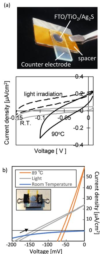
Fig. 4 The outlook and cyclic voltammogram of an Ag<sub>2</sub>S-sensitized thermal cell<sup>39</sup> (a) and a perovskite-sensitized thermal cell<sup>37</sup> (b) (Copyright © 2019 American Chemical Society).
