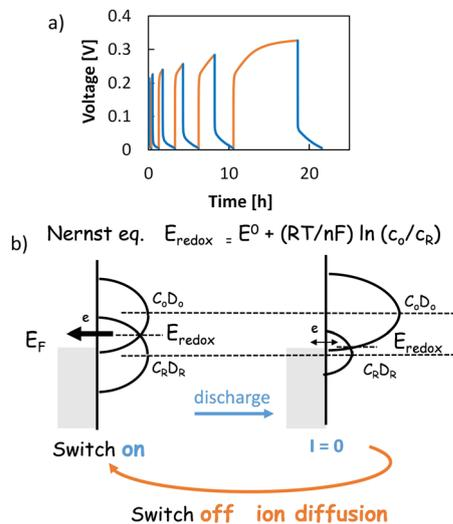
Fig. 6 Voltage behaviour of *n*-Si/Ge/copper ionic electrolyte/FTO at  $80\text{ }^{\circ}\text{C}$ ,  $100\text{ nA}$  discharge and recovery (a);<sup>45</sup> conceptual diagram of Nernst's equation (b); blue: discharge (switch on), orange: recovery (switch off).  $E_F$ : Fermi level.  $E^0$ : standard redox potential.  $c_o$ ,  $c_r$ : concentration of oxidized and reduced elements.  $D_o$ ,  $D_r$ : density of states of oxidized and reduced ions (Copyright © 2019 Royal Society of Chemistry).
