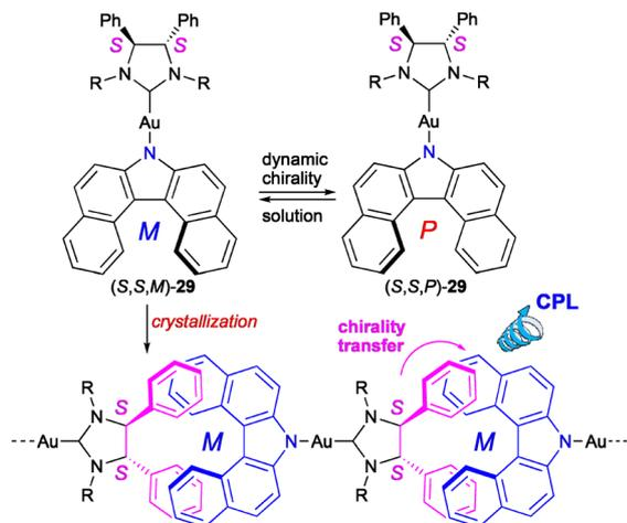
Scheme 15 Crystalline-induced chirality transfer in the aza[5]helicene Au(I) complex (S,S)-**29**. R = 3,5-di-*tert*-butylbenzyl.
