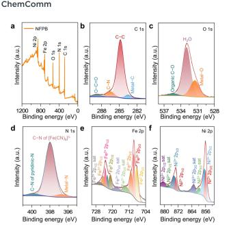
Fig. 3 (a) The XPS full spectrum of NFPB@CC. The XPS spectra of (b) C 1s, (c) O 1s, (d) N 1s, (e) Fe 2p, and (f) Ni 2p for NFPB@CC.
