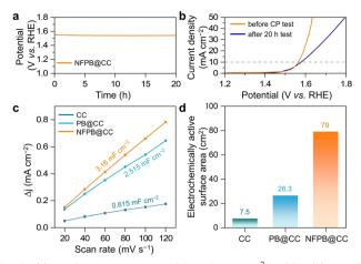
Fig. 5 (a) The CP profile of NFPB@CC at 10 mA cm<sup>-2</sup> for 20 h. (b) The LSV curve of NFPB@CC before and after the CP test. (c) The  $\Delta j$  plotted against scan rate for different samples. (d) The electrochemically active surface area of different samples
