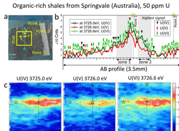
Fig. 3 (a) Photo of Springvale organic-rich shale (Australia) containing 50 ppm of U, with the selected map area of 3.5 mm (vertical)  $\times$  4.0 mm (horizontal); (b) intensity profiles along the AB line; and (c) HERFD-XRF maps showing the distribution of U(IV), U(V), and U(VI) in the selected area.
