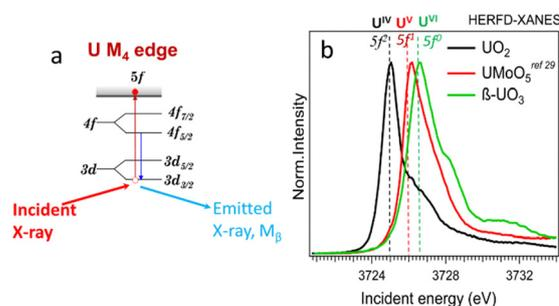
**Fig. 1** (a) Scheme of the absorption and emission processes at U M<sub>4</sub> edge, (b) HERFD-XANES spectra of U(IV), (V), and (VI) reference compounds.
