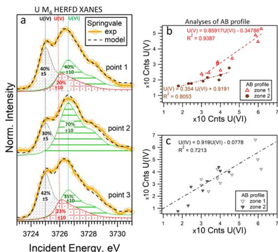
Fig. 4 (a) U  $M_4$  edge HERFD-XANES spectra measured at individual points in Springvale organic-rich shale (see Fig. 3), along with quantitative models and component contributions. The lines correspond to 3725.0 eV, 3726.0 eV, and 3726.6 eV. (b) and (c) Correlations of intensities across two regions (zone 1 and 2) of the AB profile shown in Fig. 3b. For this analysis,  $\text{UO}_2$ ,  $\text{UMoO}_5$  and  $\beta\text{-UO}_3$  were used as pure U(IV), U(v) and U(vi) references, respectively.
