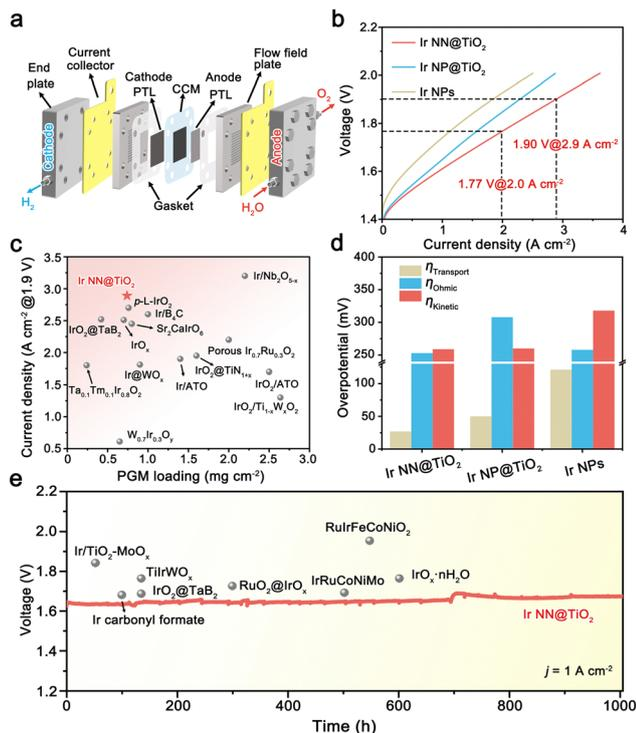
Fig. 4 (a) Schematic diagram of PEMWE. (b) Polarization curves of PEMWE using Ir NN@TiO<sub>2</sub>, Ir NP@TiO<sub>2</sub> and Ir NPs anodes. (c) Comparison of the performance of PEMWEs using different Ir-based catalysts. (d) The comparison of ohmic, transport, and kinetic losses for PEMWEs using Ir NN@TiO<sub>2</sub>, Ir NP@TiO<sub>2</sub> and Ir NPs anodes. (e) Chronopotentiometry curve of PEMWE using the NN@TiO<sub>2</sub> anode at 1 A cm<sup>-2</sup> current density.
