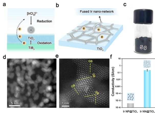
**Fig. 1** (a) Synthetic preparation of Ir NN@TiO<sub>2</sub> based on a redox reaction of H<sub>2</sub>IrCl<sub>6</sub> with TiB<sub>2</sub>. (b) Schematic illustration of Ir NN@TiO<sub>2</sub> that consists of a fused Ir nano-network on TiO<sub>2</sub> supports. (c) Digital image of 5 g Ir NN@TiO<sub>2</sub> obtained from a scaled-up synthesis. (d) and (e) TEM images of Ir NN@TiO<sub>2</sub>. (f) The comparison of the electrical conductivity for Ir NN@TiO<sub>2</sub> and Ir NP@TiO<sub>2</sub>.
