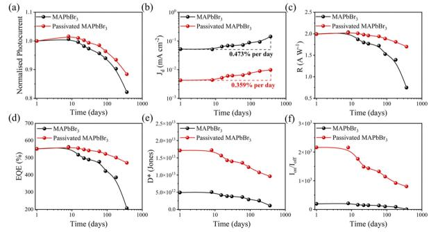
Fig. 2 Time-dependent (a) normalized photocurrent; (b) dark current density  $(J_{ph})$ , (c) responsivity (R), (d) EQE, and (e) specific detectivity ( $D^*$ ) of the control and 20 s dipped MAPbBr<sub>3</sub> SC-based PDs under a blue light of 0.1 mW cm<sup>-2</sup>. (f) Time-dependent on/off ratio of the control and 20 s passivated MAPbBr<sub>3</sub> SC-based PDs under a blue light of 50 mW cm<sup>-2</sup>
