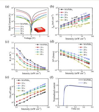
Fig. 1 (a) Dark I-V curve of the pristine MAPbBr<sub>3</sub> and passivated SC-based PDs obtained at different dipping times. (b) Photocurrent density  $(J_{ph})$ . (c) Responsivity (R), (d) specific detectivity ( $D^*$ ), and (e) on/off ratio of the pristine and passivated SC-based PDs. (f) Normalized transient photocurrent of the pristine MAPbBr $_3$  and 20 s passivated SC PDs under 1 mW cm $^{-2}$ blue light illumination at 2 V
