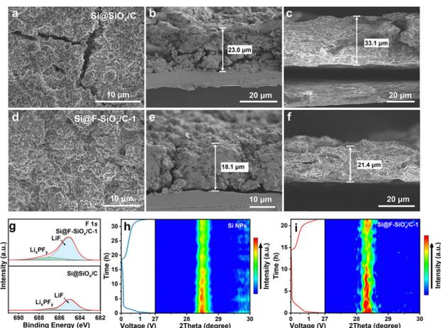
Fig. 4 Top SEM views of (a) the Si@SiO<sub>x</sub>/C and (d) the Si@F-SiO<sub>x</sub>/C-1 anode after cycling. Cross-section SEM views of (b) and (c) Si@SiO<sub>x</sub>/C and (e) and (f) Si@F-SiO<sub>x</sub>/C-1 (b) and (e) before and (c) and (f) after cycling. (g) High-resolution F 1s XPS spectra of the SEI on Si@SiO<sub>x</sub>/C and Si@F-SiO<sub>x</sub>/C-1 after cycling. *In situ* XRD pattern of (h) Si@F-SiO<sub>x</sub>/C-1 and (i) bare Si NPs during a discharge-charge cycle.
