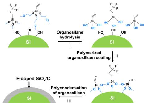
Fig. 1 Schematic illustration of the formation of Si@F-SiO<sub>x</sub>/C-1 by hydrolysis–polycondensation of VTES and TFPS on Si NPs, followed by annealing.
