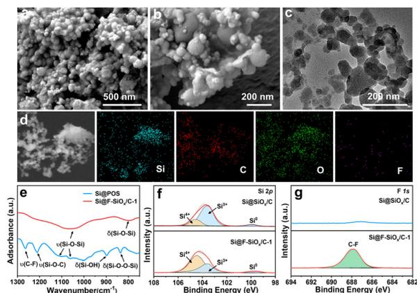
Fig. 2 (a) and (b) SEM and (c) TEM image of Si@F-SiO<sub>x</sub>/C-1 consisting of interconnected NPs. (d) Elemental mapping showing the uniform dispersion of Si, C, O, and F elements within Si@F-SiO<sub>x</sub>/C-1. (e) FT-IR spectra of Si@F-SiO<sub>x</sub>/C-1 and Si@POS. (f) High-resolution XPS spectra for (f) Si 2p and (g) F 1s signals of Si@F-SiO<sub>x</sub>/C-1 and Si@SiO<sub>x</sub>/C.
