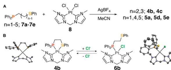
**Fig. 1** (A) Synthesis of bis-carbene hemilabile ligand Pt(II) complexes. (B) Reversible  $\text{Cl}^-$ -promoted structural interconversion of **4b** and **6b** and their crystal structures drawn with 50% probability ellipsoids. Counterions, hydrogens, and solvent molecules are omitted for clarity (C: gray, P: orange, S: yellow, N: purple, Pt: white, Cl: green).
