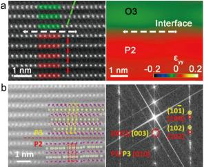
Fig. 4 (a) STEM-HAADF image of the O3/P2 hybrid composite of the O3/ P2  $a_{0.8}[Ni_{0.5}Co_{0.2}Mn_{0.3}]O_2/Na_{0.8}[Ni_{0.33}Mn_{0.67}]O_2$  cathode with corresponding strain mapping. Reproduced with permission from ref. 50, copyright 2020 American Chemical Society. (b) STEM-HAADF image of a P2/P3 biaphase Na<sub>0.67</sub>Mn<sub>0.64</sub>Co<sub>0.30</sub>Al<sub>0.06</sub>O<sub>2</sub> particle with corresponding FFT patterns. Reproduced with permission of ref. 41, copyright 2021 Wiley.
