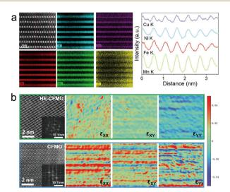
Fig. 5 (a) STEM-EDS mapping of O and TM elements, Ni (cyan), Cu (purple), Fe (red), and Mn (green) of the HE layered oxide Na<sub>0.95</sub>Li<sub>0.06</sub>- $Ni_{0.25}Cu_{0.05}Fe_{0.15}Mn_{0.49}O_2$ , with corresponding line profiles across the layers. Reproduced with permission from ref. 64, copyright 2023 Springer Nature. (b) STEM-HAADF images and the corresponding GPA analysis results of HE-CFMO and CFMO cathodes. Reproduced with permission from ref. 64, copyright 2024 Wiley.
