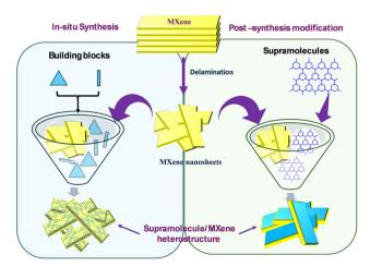
Fig. 6 Synthesis of heterostructures via in situ and post-synthesis
