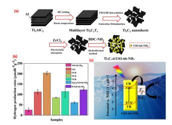
Fig. 11 (a) Synthesis scheme of the TU series; (b) H<sub>2</sub>-generation rates under photocatalytic conditions of samples; and (c) proposed mechanism. Reprinted with permission from ref. 29 Copyright 2019 Elsevier.
