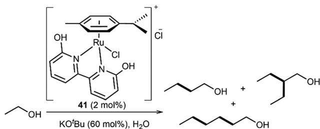
**Scheme 8** A water-soluble ruthenium catalyst **41** used for the upgrading of ethanol.<sup>96</sup>
