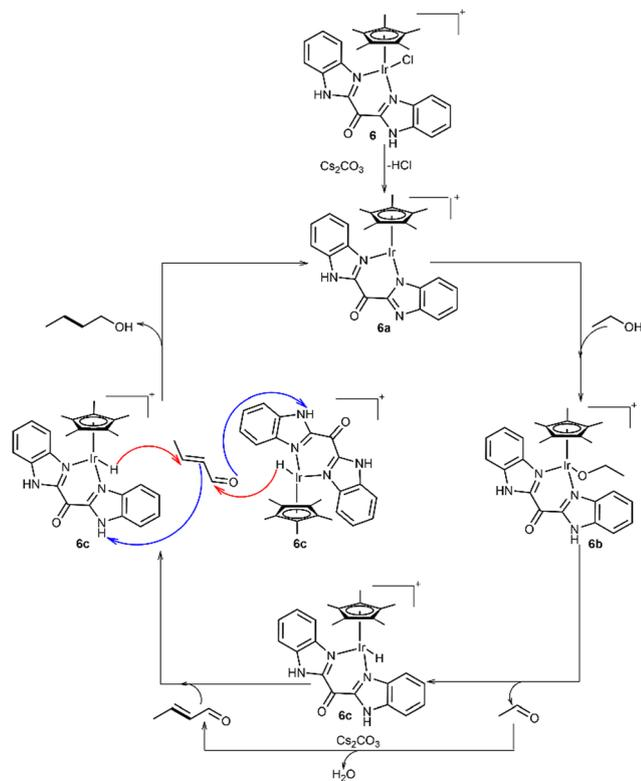
Fig. 5 Plausible mechanism proposed by Li and co-workers for ethanol upgrading using a Cp\*Ir-based catalyst.<sup>74</sup>
