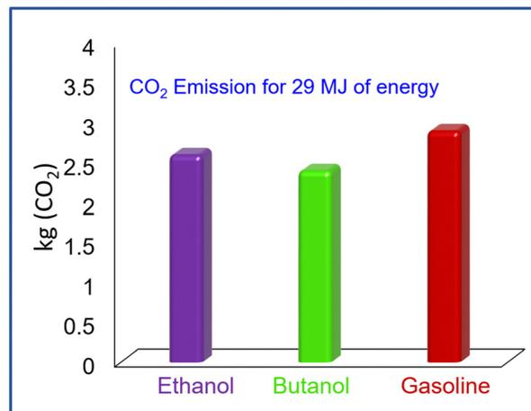
Fig. 2 Comparison of CO<sub>2</sub> emissions from gasoline, butanol, and ethanol while generating 29 MJ of energy.<sup>13</sup>
