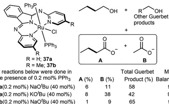
Fig. 11 Pincer–Ru complexes used for ethanol upgrading by Szymczak and co-workers.<sup>87</sup>
