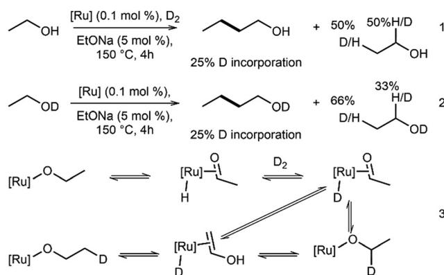
Scheme 4 Mechanistic insights into the ruthenium-catalysed Guerbet reaction, as proposed by Wass and co-workers.<sup>79</sup>
