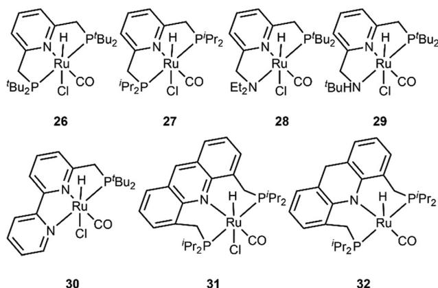
Fig. 8 Pincer ruthenium catalyst reported for ethanol upgrading by Milstein and co-workers.<sup>82</sup>
