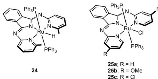
Fig. 7 Pincer–ruthenium catalysts reported for ethanol upgrading by Szymczak.<sup>81</sup>
