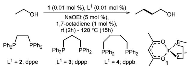
Scheme 2 First example of the Guerbet reaction catalyzed by the homogeneous Ir-complex.<sup>71a</sup>
