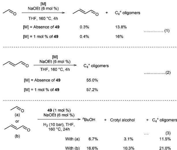
Scheme 10 Mechanistic studies performed by Q. Liu during the 49-catalysed upgrading of ethanol to higher alcohols.<sup>100</sup>
