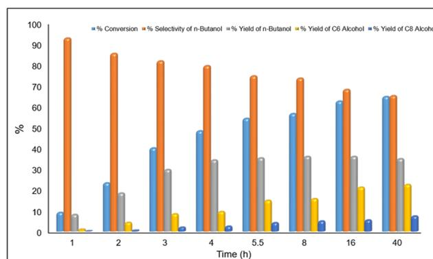
Fig. 9 Reaction profile for the **31**-catalysed ethanol upgrading reaction reported by Milstein and co-workers.<sup>82</sup>
