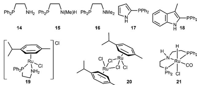
Fig. 6 Combination of mixed ligands and ruthenium complexes used by Wass and co-workers for the Guerbet reaction.<sup>80</sup>
