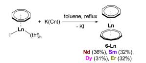
Scheme 5 Synthesis of the heteroleptic sandwich complexes [(Cnt)Ln|||- $(\eta^8-\text{Cot})$ ] (6-Ln, Ln = Nd, Sm, Dy and Er) from  $[(\eta^8-\text{Cot})\text{Ln}^{||}](\text{thf})_n]$ and K(Cnt).
