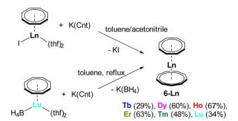
Scheme 6 Synthesis of the heteroleptic sandwich complexes [(Cnt)Ln<sup>III</sup>( $\eta^8$ -Cot)] (**6-Ln**, Ln = Tb, Dy, Ho, Er, Tm and Lu) from  $[(\eta^8-\text{Cot})\text{Ln}^{|||}]$  (Tb, Dy, Ho, Er, and Tm) and K(Cnt) in toluene/ acetonitrile mixture or from  $[(\eta^8-Cot)Lu^{III}(BH_4)(thf)_2)]$  and K(Cnt) in toluene under reflux.
