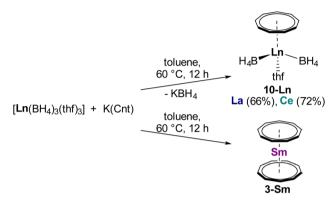
Scheme 10 Synthesis of the half sandwich complexes 10-Ln and reaction between [Sm<sup>III</sup>(BH<sub>4</sub>)<sub>3</sub>(thf)<sub>3</sub>] and K(Cnt).
