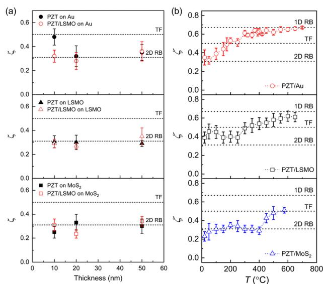
Fig. 7 DW roughness in PZT membranes. (a)  $\zeta$  vs. PZT thickness at room temperature for PZT and PZT/LSMO membranes on different base layers. (b)  $\zeta$  vs. TQ temperature for 50 nm PZT membranes on different base layers. Reproduced from ref. 28 with permission from American Chemical Society, copyright 2023.
