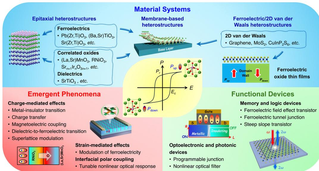
Fig. 1 Overview of research on ferroelectric perovskite oxide-based heterostructures, including material systems, emergent phenomena, and potential device applications.  $P_{up}/P_{down}$ : polarization up/down.
