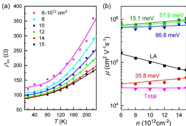
**Fig. 18** Effect of RSO phonons on a BSTO-gated 1L graphene FET. (a)  $\rho_{xx}(T)$  at various hole doping levels with fits to eqn (3). (b) Mobility limit at 300 K imposed by the LA and four RSO phonon modes and the overall contribution (total). Reproduced from ref. 149 with permission from AIP Publishing, copyright 2022.
