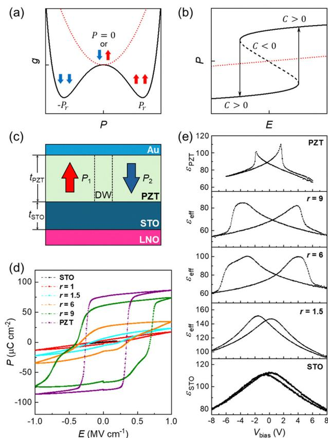
**Fig. 14** FE-to-DE transition in PZT/STO stacks. (a) and (b) Schematics of ferroelectric free energy density  $g$  vs.  $P$  (a) and  $P$ - $E$  loop (b). The dotted lines represent the dielectric responses. (c) Schematic of a PZT/STO stack hosting a DW. (d)  $P$ - $E$  loops and (e) effective dielectric constant vs.  $V_{\text{bias}}$  for PZT/STO stacks with different PZT/STO thickness ratios  $r$ . Reproduced from ref. 39 with permission from American Physical Society, copyright 2021.
