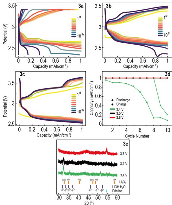
**Fig. 3** Constant current constant voltage protocol with redox mediator. (a)–(c) CCCV potential curves of Li–O<sub>2</sub> cells containing Lil as a redox mediator in the electrolyte cycled at a range of upper-cut-off voltages (UCVs); (a) 3.4 V, (b) 3.5 V and (c) 3.8 V. (d) Discharge and charge capacity per cycle comparison. (e) XRD patterns of electrodes taken after the 10th discharge–charge cycles.
