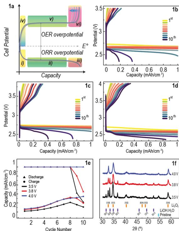
**Fig. 1** Constant current protocol. (a) Typical galvanostatic cycling (CC) potential curves of Li–O<sub>2</sub> cells. (b)–(d) CC potential curves of Li–O<sub>2</sub> cells cycled at a range of upper-cut-off voltages (UCVs); (b) 3.5 V, (c) 3.8 V, and (d) 4.0 V. (e) Discharge and charge capacity per cycle comparison. (f) XRD patterns of electrodes taken after the 10th discharge–charge cycles.
