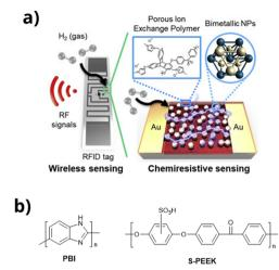
Fig. 17 (a) Polymer-based RFID sensors (Copyright CelPress 2020), <sup>97</sup> and (b) chemical structure of PBI and S-PEEK.
