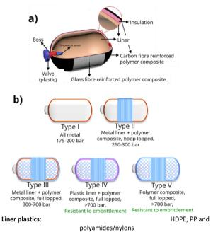
phenolics, polyamides and polyphenylene sulphide. Fig. 13 (a) General structure of a vehicle on-board high-pressure hydrogen storage tank (copyright ACS 2023), 69 and (b) different types of hydrogen storage tanks. Liner plastics: HDPE, PP and polyamides/nylons.
