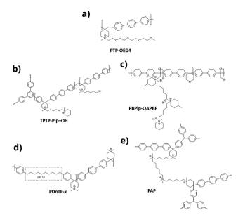
**Fig. 16** Chemical structure of (a) PTP-OEG4, (b) TPTP-Pip-OH, (c) etherfree fluoropolymer PBPip-QAPBF, (d) poly(aryl-co-terphenyl piperidinium) based AEMs PDnTP-x and (e) poly(aryl piperidinium) (PAP) based anion exchange membranes.
