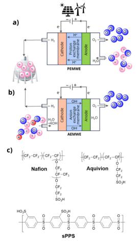
Fig. 3 (a) Proton exchange membrane water electrolysers (PEMWEs), (b) anion exchange membrane water electrolysers (AEMWEs) and (c) chemical structure of Nafion, Aquivion and sulfonated poly(phenylene sulfone) (sPPS) used as membrane materials
