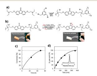
(a) Synthesis of fluoreneone polymer, (b) dehydrogenated and hydrogenated forms of fluorenone (orange)-fluorenol (white) polymer sheets, (c) hydrogenation kinetics of fluorenone polymer at 25 °C and 1 atm of hydrogen gas and (d) dehydrogenation kinetics of fluorenol polymer at 95 °C (inset gas chromatography plot of the hydrogen peak).<sup>52</sup> Copyright Wiley 2020
