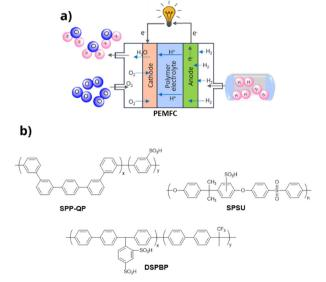
Fig. 15 (a) A proton exchange membrane fuel cell (PEMFC), and (b) chemical structures of some of the sulfonated polymers used as fuel cell membranes.
