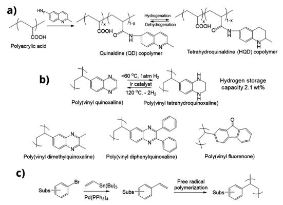
Fig. 10 (a) Quinaldine copolymer, (b) homopolymers from quinoxaline derivatives and fluorenone used for hydrogenation–dehydrogenation studies and (c) the usual synthesis protocol of monomer and polymer synthesis of quinoxaline and fluorenone.
