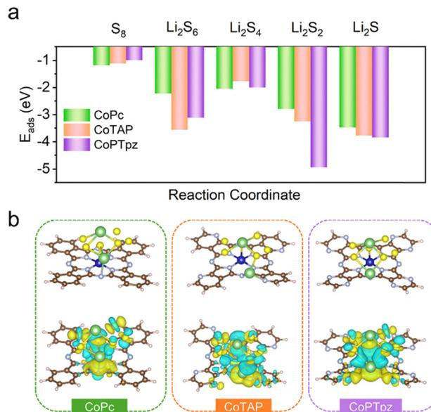
Fig. 3 (a) The adsorption energies of all optimized structures. (b) The electron density differences of CoPc, CoTAP and CoPTpz with  $Li_2S_6$ . The blue and yellow regions indicate the accumulation of positive and negative charges, respectively.
