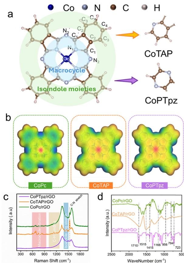
**Fig. 1** (a) The atomic structures of CoPc, CoTAP, and CoPTpz. (b) The corresponding surface electrostatics. (c) The Raman spectra of CoPc/rGO, CoTAP/rGO and CoPTpz/rGO. (d) The FTIR spectra of CoPc/rGO, CoTAP/rGO and CoPTpz/rGO.
