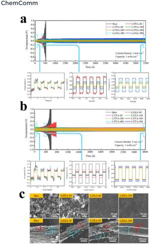
Fig. 4 The effect of LiTEA-coating on Li-metal electrodes at different current densities (a) 2 and (b) 5 mA cm<sup>-2</sup> at a fixed areal capacity of 1 mA h cm<sup>-2</sup>. (c) The SEM images of Li electrode surfaces (top images) and electrode cross-sections (bottom images) for bare and coated Li electrodes after 500 Li-stripping/plating cycles at 2 mA cm<sup>-2</sup> and 1 mA h cm<sup>-2</sup>. Adapted with permission from ref. 54. Copyright 2023, Chemical Engineering Journal.
