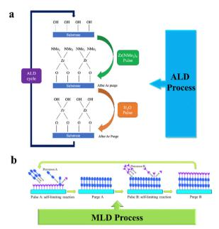
Fig. 1 (a) Schematic illustration of the ALD deposition of zirconium oxide (ZrO<sub>2</sub>) using TDMA-Zr and H<sub>2</sub>O as precursors. Adapted with permission from ref. 21. Copyright 2020, Materials Research Society. (b) Schematic illustration of a general MLD process using two homobifunctional organic precursors of A and B. Adapted with permission from ref. 18. Copyright 2024, Inorganic Chemistry Frontier.
