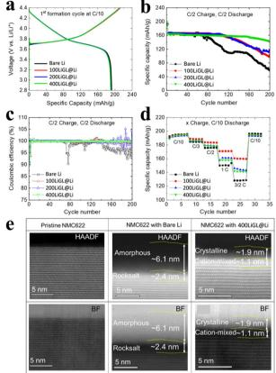
Fig. 3 The effects of LiGL-coated Li anodes on Li NMC622 cells. (a) The first charge/discharge profiles of full cells with bare Li and LiGL-coated-Li coupled with NMC622 (1C =  $4.2 \text{ mA cm}^{-2}$ ). For different thicknesses of the Li coating at 2.8-4.4 V, (b) cyclability at C/2, (c) CE at C/2, (d) C-rate, and (e) HAADF and BF images of pristine NMC622 coupled with coated and uncoated Li. Adapted with permission from ref. 52. Copyright 2024, Small Structures
